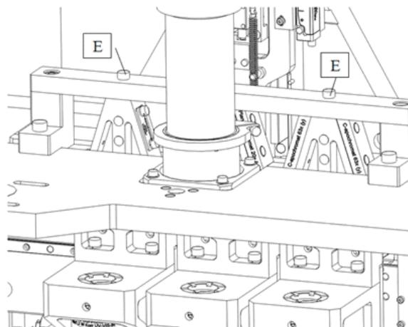
**Figure 33 – Mount fixing blocks on objective changer**
