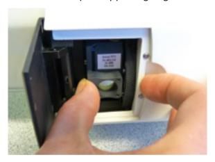
Figure 84 – Positioning the filter cube
