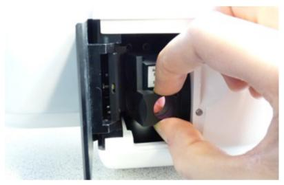
Figure 85 – Removing the filter cube
