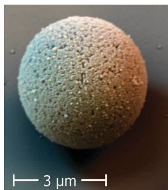
Figure 1. Scanning electron micrograph of Dynabeads magnetic beads. The nonporous, uniform nature of the beads enable low nonspecific binding, high reproducibility, low antibody consumption, and fast binding kinetics.
