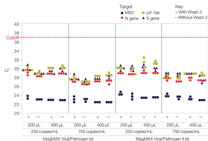
Figure 1. C_t values for contrived SARS-CoV-2-positive nasopharyngeal swab samples with different sample preparation workflows. Nasopharyngeal swab specimens were spiked with 250 copies/mL or 750 copies/mL of SARS-CoV-2 viral RNA (1x or 3x the limit of detection, respectively), and RNA was extracted from 200 \mu\text{L} or 400 \mu\text{L} of the spiked sample in triplicate using either the MagMAX Viral/Pathogen or MagMAX Viral/Pathogen II kit with or without Wash 3. After elution in 50 \mu\text{L} , the samples were assayed by qRT-PCR. All negative samples had C_t values of “Undetected” (data not shown).
