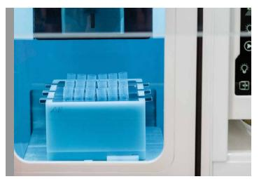
Figure 3. The sort collector with numerous sort tubes.
