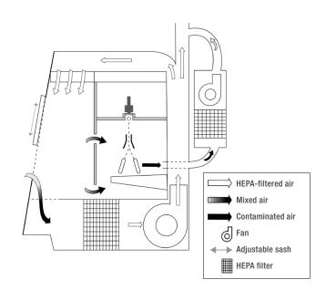
Figure 1. Airflow diagram.
