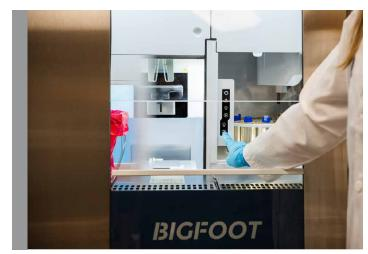
Figure 4. The internal control panel that limits the need for the operator to reach in and out of the enclosure.
