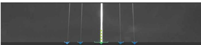
Figure 3. Test pattern with alignment targets of four-way plate sorting mode for 384-well plates.
