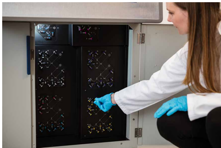
Figure 26. PMTs and filters on the Bigfoot Spectral Cell Sorter.
