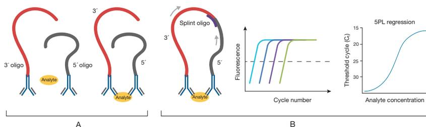
**Figure 2. How ProQuantum immunoassays work.** (A) Antibody conjugates bind to target during a 1 hr incubation. (B) With addition of a splint oligonucleotide and DNA ligase, the two antibody-conjugated oligonucleotides are ligated to create a 100-base template that is amplified through 40 qPCR cycles. The amount of DNA produced, measured via fluorescence, is directly proportional to the number of amplicons generated.
