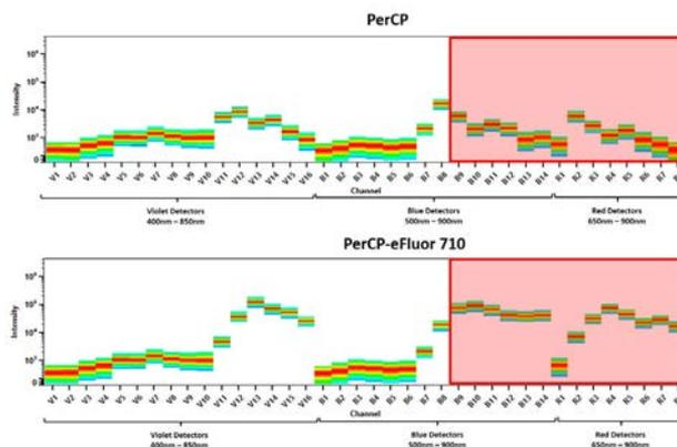
Comparison of cells labeled with PerCP and the tandem fluorophore PerCP-eFluor 710. Although the emission profiles are similar, the unique patterns in the far-red channels allow for the two fluorophores to be discriminated using spectral flow cytometry.
