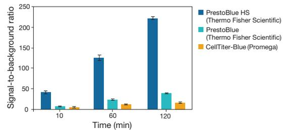
**Sensitivity comparison between conventional cell viability reagents and the new alamarBlue HS and PrestoBlue HS reagents.** A549 cells were assayed with the indicated cell viability reagents according to the manufacturers' protocols. Resorufin fluorescence was measured using the Thermo Scientific™ Varioskan™ LUX Multimode Microplate Reader.
