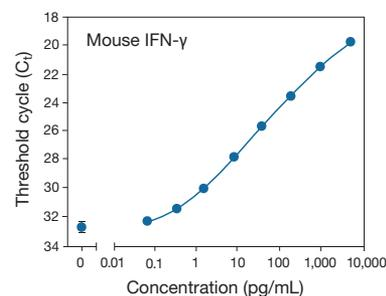
**Standard curve for the IFN gamma Mouse ProQuantum Immunoassay Kit.** This standard curve shows an assay range of 0.064–5,000 pg/mL.
