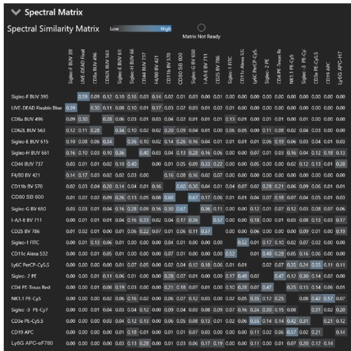
**Figure 3. Spectral similarity matrix.** The spectral similarity matrix (with values of 0–1.0) of SQ Software allows the user to identify fluorophore combinations that cause an increase in complexity and may be more difficult to spectrally unmix.
