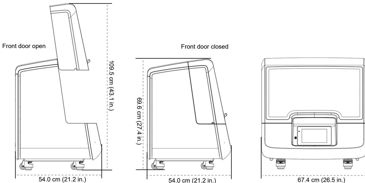
**Figure 1** Instrument dimensions
