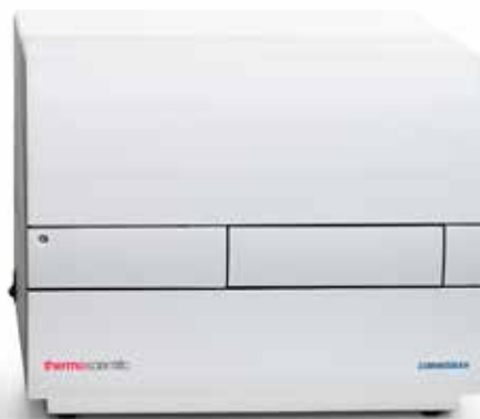
Luminoskan microplate reader— dedicated luminometer
