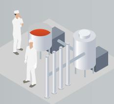
FBS is transferred to a cleanroom in specially designed stainless steel pipes where it undergoes 0.1 µm triple filtration to minimize biological contaminants.
