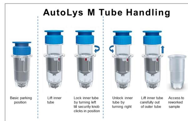
FFPE samples (curls, slides, cores) are placed in the tubes and protease digestion happens directly in them. After digestion is complete, the tubes are lifted from parking to the centrifuge position. Samples are spun allowing a physical separation of wax and tissue. Tubes are lifted to a final position so the lysate can be accessible for purification.
