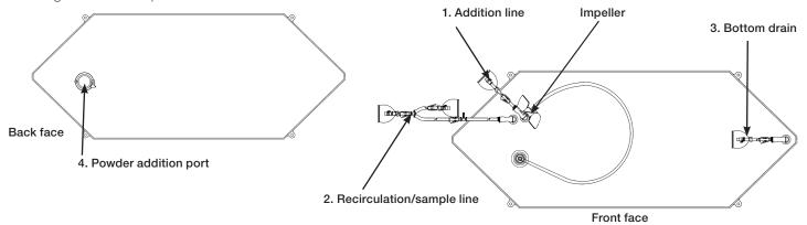
Standard 2,000 L BPC for powder-to-liquid applications without probe ports
