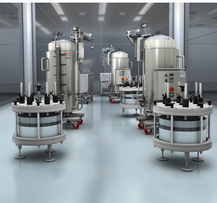
Figure 1: Downstream processing of biological products using large scale chromatography.
