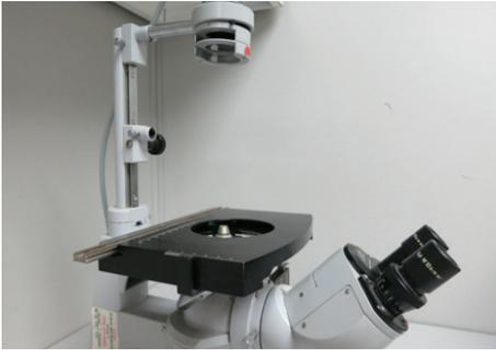
Begin by removing all stage accessories to provide a flat surface for the Cell Factory system to rest upon. If additional space is required, remove the light source.
