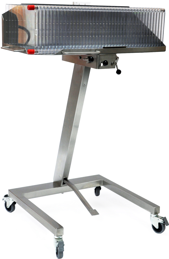
40-layer Nunc Cell Factory hand manipulator system
