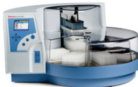
Pharma KingFisher Flex 96 Deep-Well Magnetic Particle Processor 192 extractions per day
