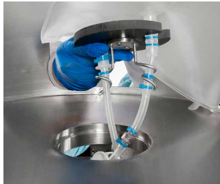
Figure 5. Sparge line support.
