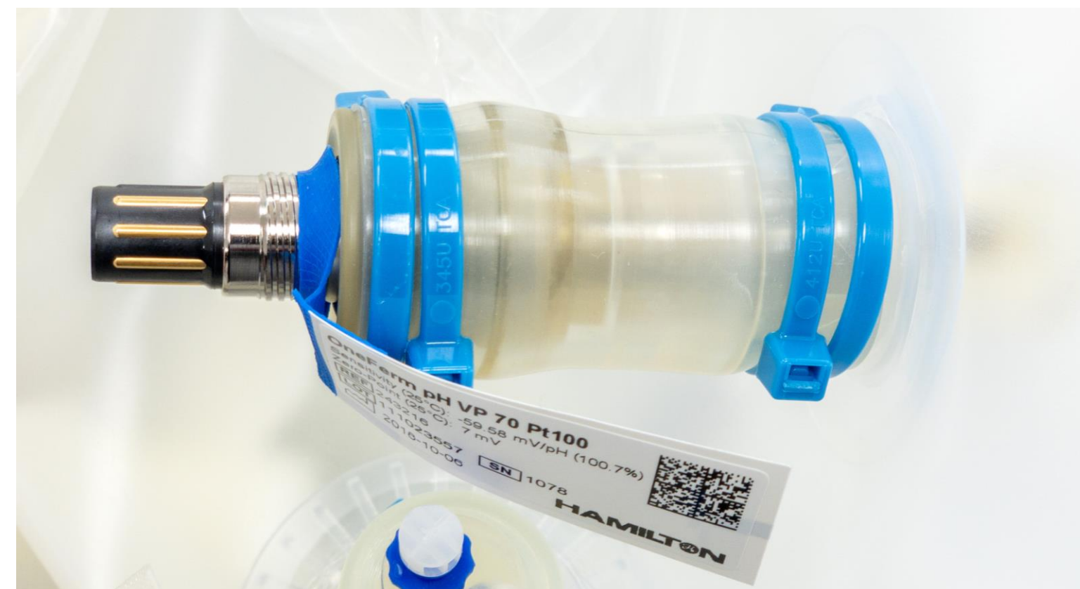
Figure 1. Image of OneFerm™ sensor installed in a S.U.B. BPC
