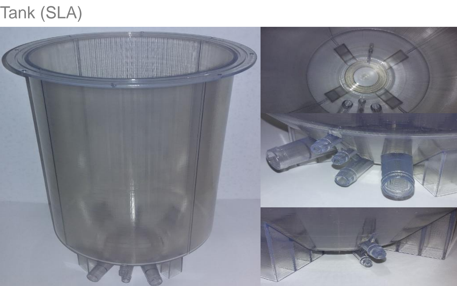
Figure 2. Photos of bioreactor parts that have been manufactured using different rapid prototyping techniques
