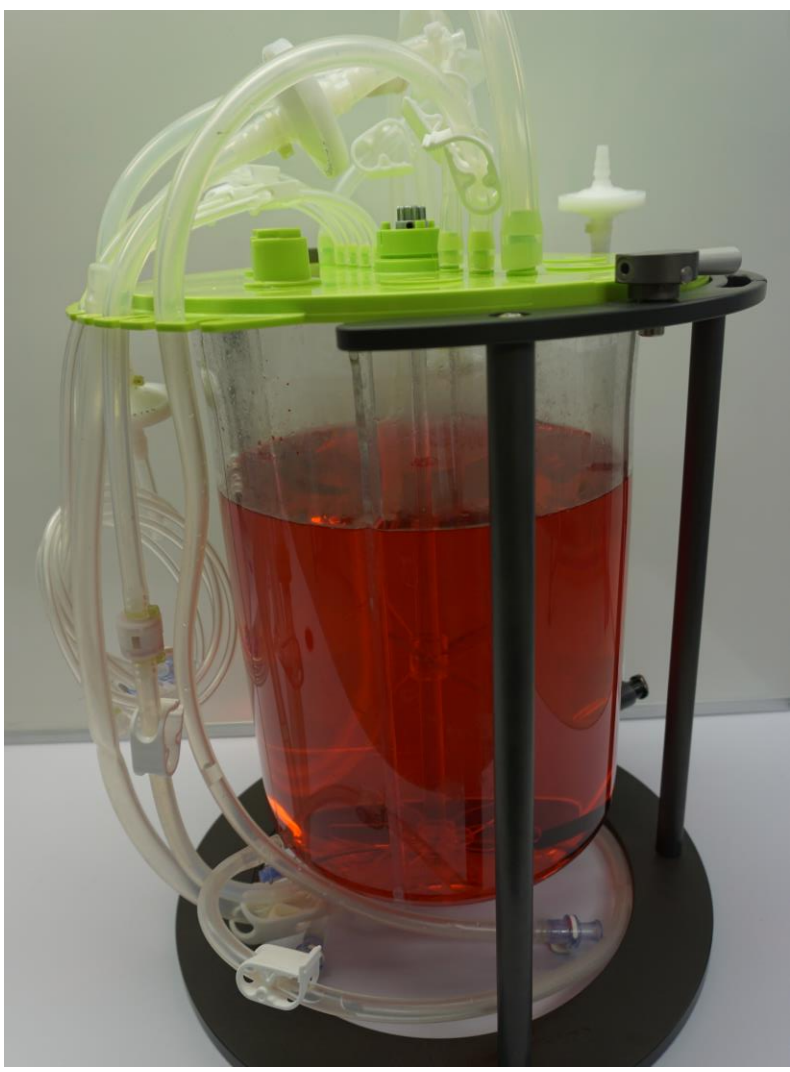
Figure 8. Picture of a final prototype made by injection molding that is placed in a vessel stand for operations
