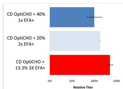
Leveraging super-concentrated feeds can improve bioreactor operations and increase titer:
