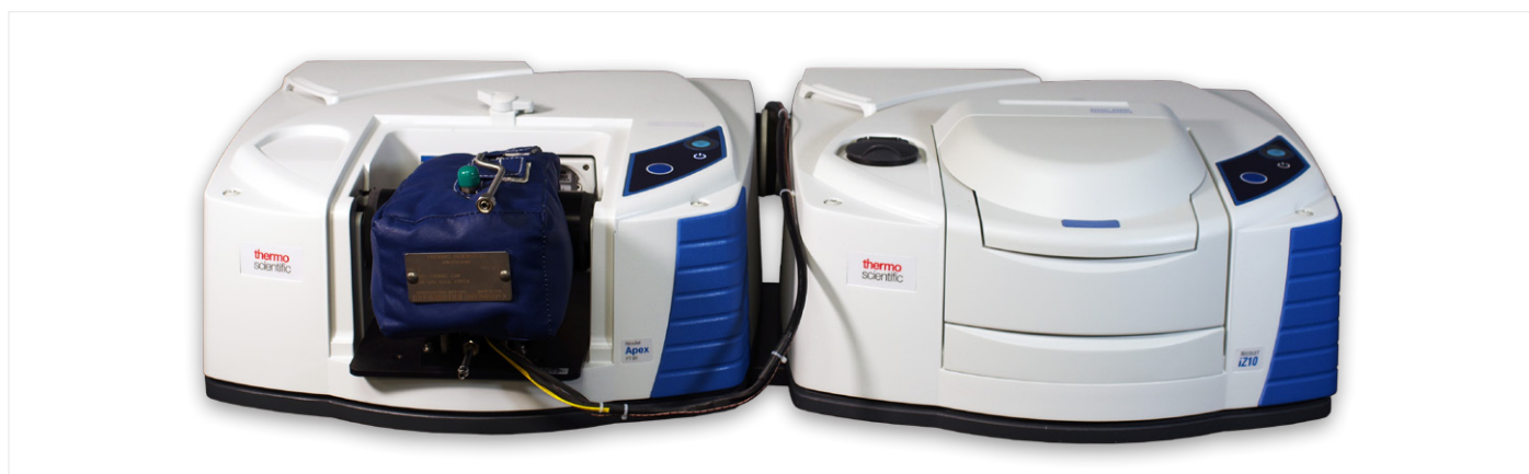
Figure 3. Photo of a Thermo Scientific Nicolet Apex FTIR Spectrometer equipped with a TEC-MCT detector. The 2-m gas cell is in the main sample compartment. The iZ10 module is configured with a smart iTX ATR and DTGS-KBr detector. The setup allows for easy switching between accessories and detectors.
