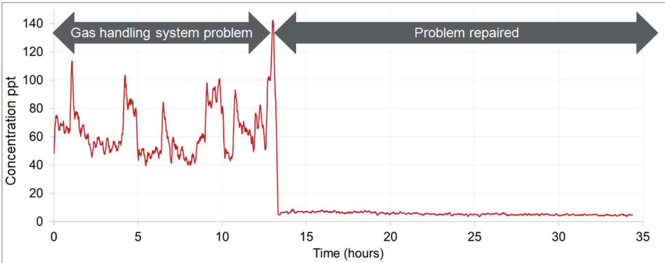
Figure 2. APIX analysis of methane impurity in argon
