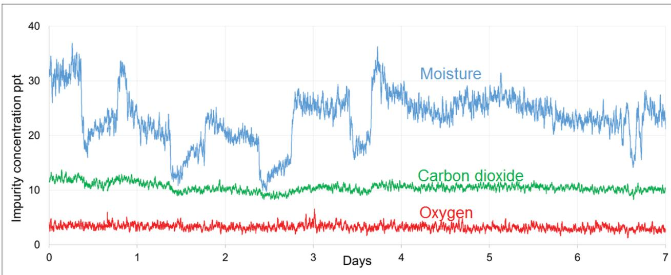
Figure 3. APIX analysis of moisture, carbon dioxide and oxygen in nitrogen
