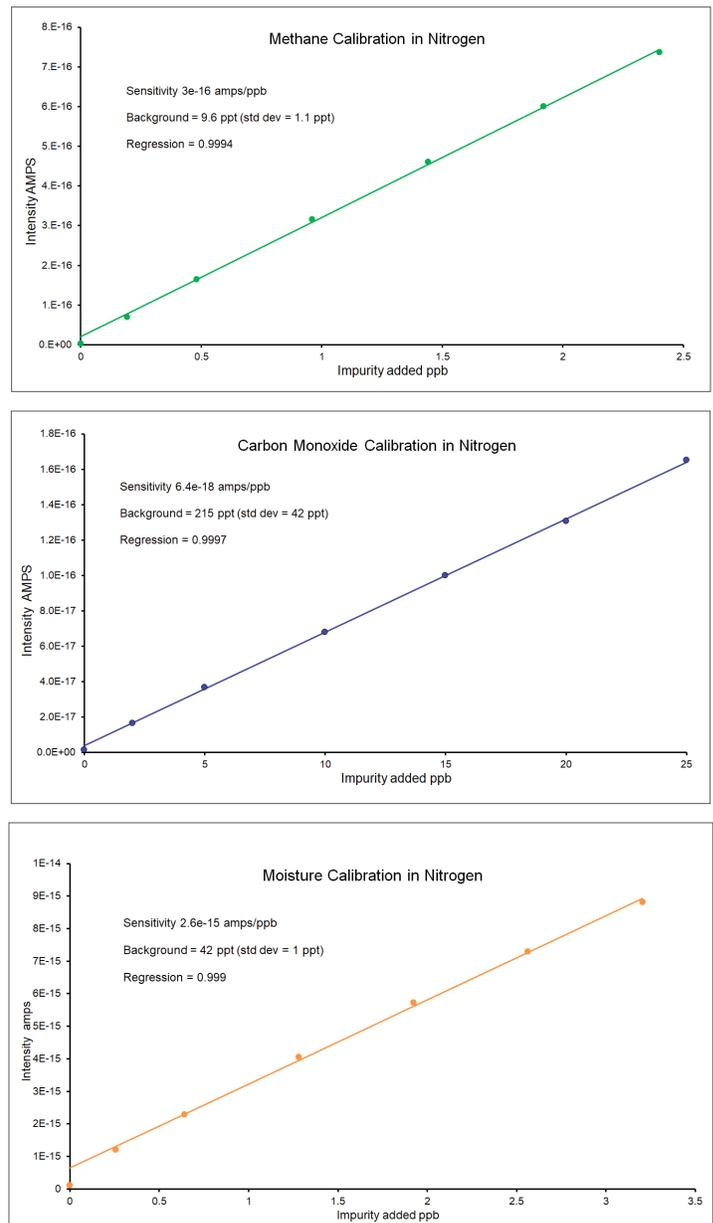
**Figure 6. Linearity plots for methane, carbon monoxide and moisture generated by the APIX gas processor.**
