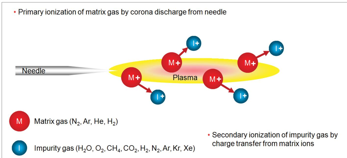
Figure 1. API charge transfer for bulk matrix gas to trace impurities
