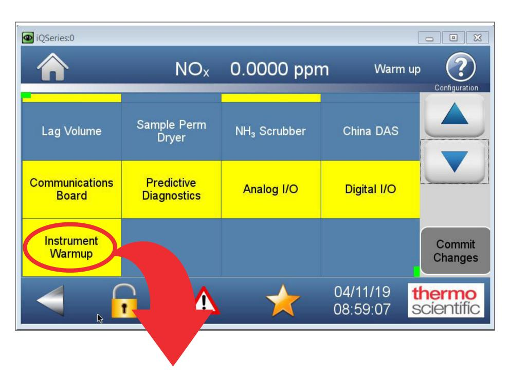
You can now disable the **Warm-up** feature in the instrument's Configuration menu. Remember, concentration readings are not accurate until the instrument stabilizes and is **Alarm FREE**.
