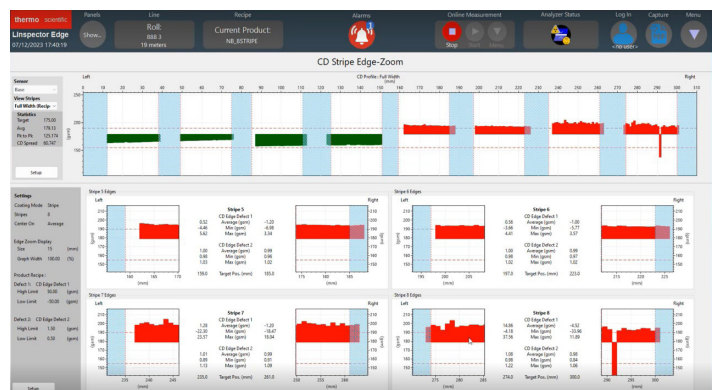
Figure 5. CD stripe edge zoom profiles showing sub-zoom windows for each edge (lower half of the image)
