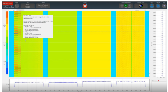
Figure 4. Heat map view with edge defect identification
