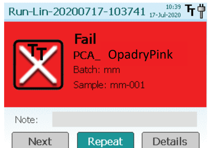
Figure 4: Pass or Fail Screen Display of PCA model for verification of raw materials. Detailed chemometric results are also shown on the screen.
