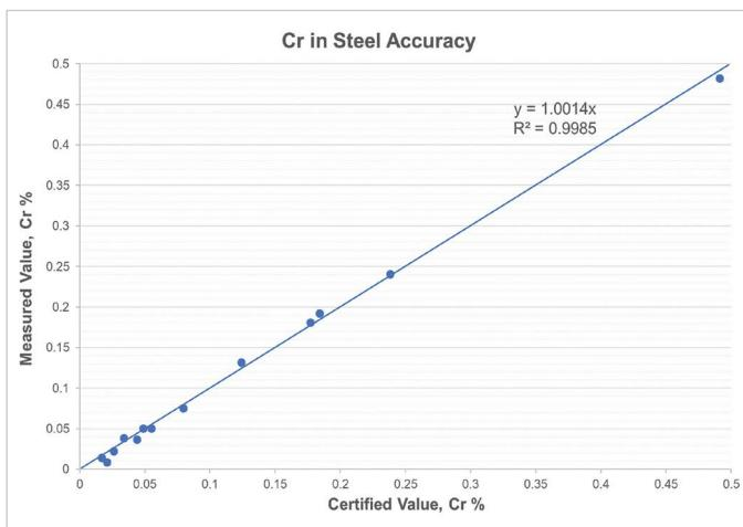
Figure 1: Chromium in steel accuracy using the Niton XL5 Plus analyzer
