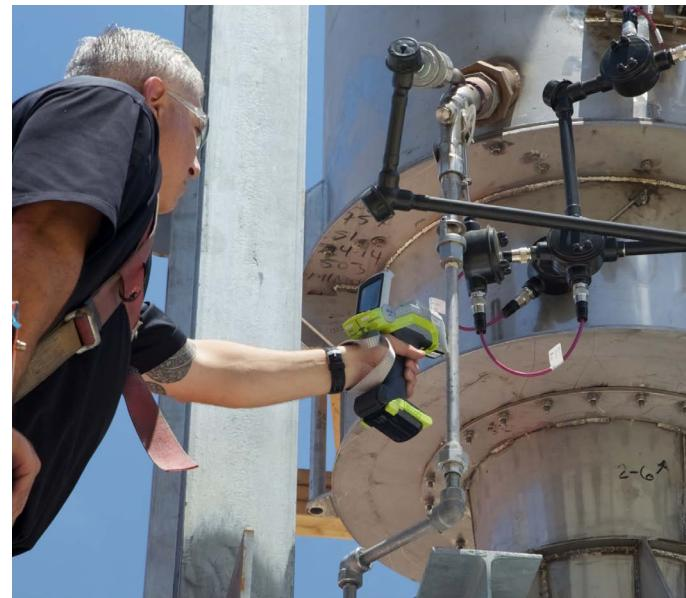
An inspection is conducted using the handheld Niton XL5 Plus XRF analyzer.
