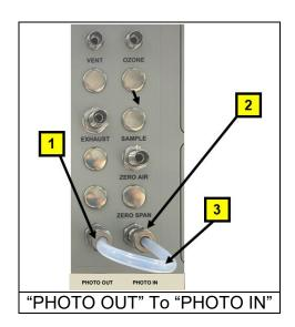
2. To sample external ozone (generated by a device other than the 49iQPS), remove (and save) your short jumper hose. Install a ¼" Stainless plug/cap on the "PHOTO OUT" port. Connect your external ozone to the "PHOTO IN" port.
