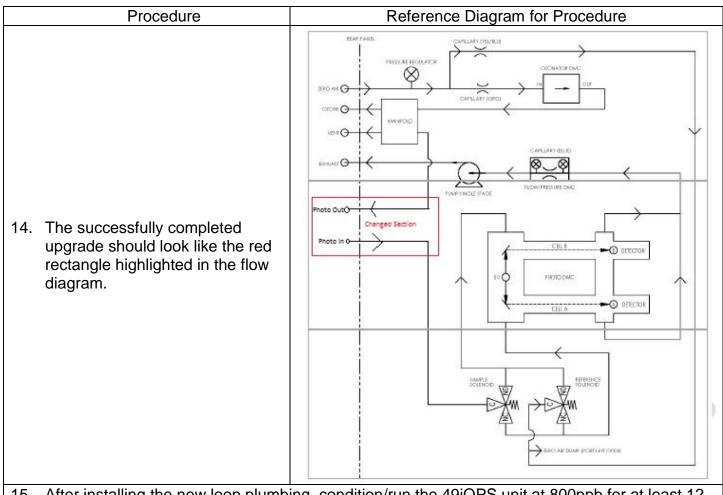
15. After installing the new loop plumbing, condition/run the 49iQPS unit at 800ppb for at least 12 hours.
