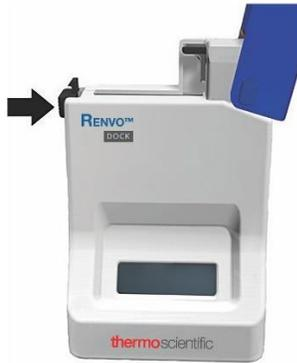
3. Insert the Test Cassette into the slot with the cassette label facing the front of the Dock. The sample port (covered with a foil tab) on the top of the cassette is accessible to you. Fully press the Test Cassette into the Dock until it 'clicks' into position. The Renvo Dock measures the temperature of the cassette and displays it as shown in the example below:
