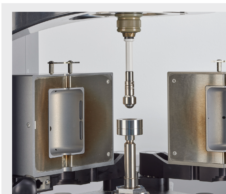
Figure 3: Temperature-dependent tribo-rheological measurements using the temperature chamber for HAAKE MARS iQ Rheometer series. 3
