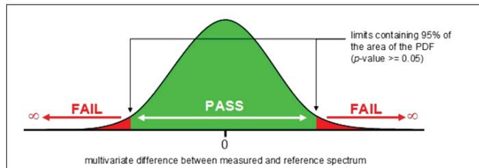
Figure 3. TruScan RM pass/fail univariate t-distribution.
