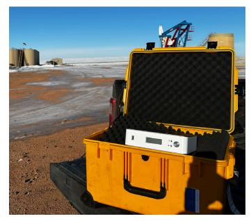
A solid-state Raman spectroscopy system, the MarqMetrix All-In-One Process Raman Analyzer has no moving parts, making it ideal for continuous process monitoring, including in-line, at-line, or off-line and routine laboratory analysis.
