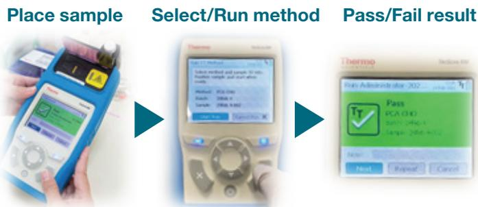
Figure 1. Workflow for Raman spectroscopy analysis.
