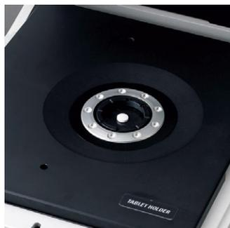
With its iris format, the Tablet Holder accepts tablets in a range of sizes.
