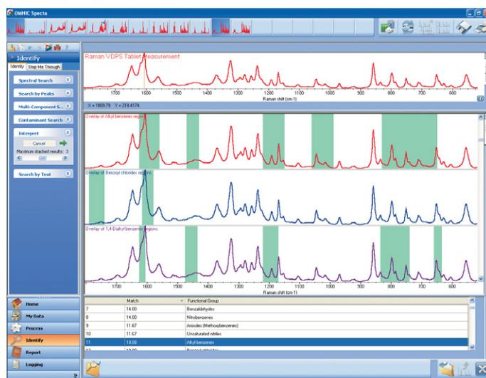
In a single step, OMNIC Specta determines the identify of the three active ingredient in a multicomponent table: acetaminophen, acetylsalicylic acid, and caffeine.
