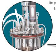
to 350 degrees Celsius. MarqMetrix BallProbe Sampling Optics are also available in bioreactor-specific versions with a seal and nut to allow for immersion in a reaction vessel, be it a dedicated stainless-steel bioreactor or a single-use bioreactor. These Thermo Scientific™ MarqMetrix™ Bioreactor BallProbe™ Sampling Optics are autoclavable, either while attached to the bioreactor, or on their own when cleaning and sterilizing the ball probe separately.
