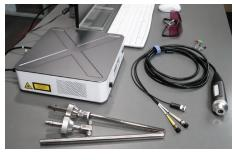
MarqMetrix All-In-One Process Raman Analyzer is compact. With a footprint less than one square foot and three inches tall, MarqMetrix
