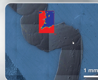
Marker on polymer with IR analysis.
