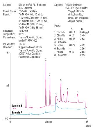
Figure 1. Analysis of trace anions in high-purity water with capillary ion chromatography.
