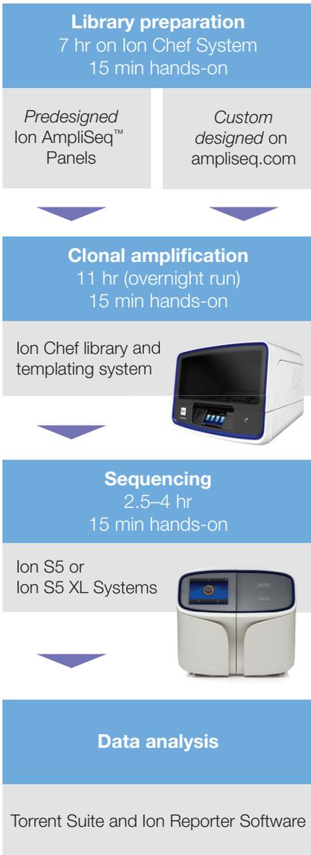
**Figure 2. Targeted sequencing workflow.** Ion AmpliSeq libraries are prepared manually or with the Ion Chef System. Libraries are then placed in the Ion Chef System for emulsion PCR, enrichment, and loading onto Ion chips. Chips are placed in the Ion S5 System with reagents for sequencing. Primary data analysis is performed by Torrent Suite Software.
