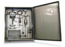
Housed in a stainless steel enclosure, the basic Sarasota SG901 system comprises a Thermo Scientific Sarasota FD900 gas density assembly, temperature element, and flow control valve. All components are binterconnected by 6.35 mm (0.25") stainlessbsteel tubing. The basic system is ideal for applications where the analyzer is used in conjunction with an existing gas conditioning system that provides a clean, dry sample at a pressure below 4 bar A (58 psia).
