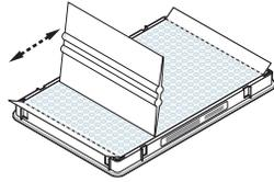
6. Use the applicator to hold the edge of the film in place, then grasp one end of the tab and sharply pull up and away. Repeat the action to remove the other tab.
