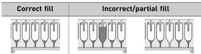
If necessary, centrifuge the cards for an additional minute to fill any unfilled wells. Do not exceed three 1-minute runs or centrifuge the card for longer than 1 minute at a time.
