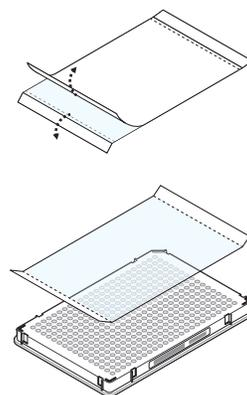
5. While applying firm downward pressure, move the applicator slowly across the film, both horizontally and vertically, to ensure good contact between the film and the entire surface of the reaction plate.
