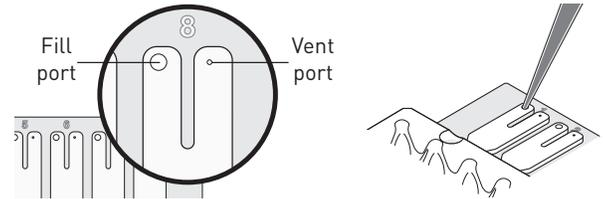
d. Dispense the fluid so that it sweeps in and around the fill reservoir toward the vent port.
