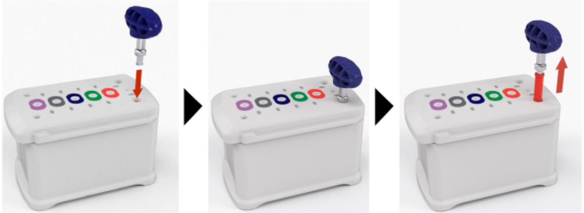
4. Remove the scrubber from the cartridge tool, then discard the scrubber according to applicable hazardous waste regulations.
