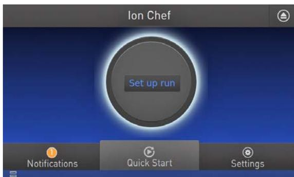
3. Tap **Step by step** to have the instrument lead you through the instrument setup, or tap **Quick Start** to skip the instrument setup screens and proceed to Deck Scan.
