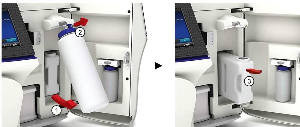
3. Reinstall the empty waste reservoir and a *used* Ion S5™ Wash Solution bottle.
