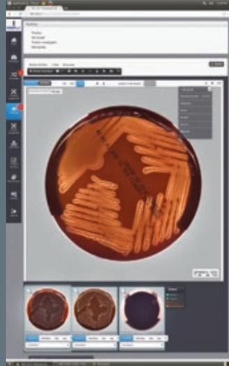
*Bottom light no background— Simulates holding to the light to see hemolysis*
