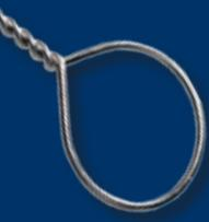
**MICROBIOLOGY LABS** have always used traditional loops. Seeing no point in trying to change what has always worked, WASP®DT uses reusable metal loops ranging in size from 1µl, 10µl and 30µl. Other automated systems use pipet tips, which cannot transfer volumes less than 10µl, and the difference is clear.
