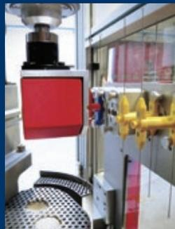
Automatically switch between 1µl, 10µl or 30µl loop
