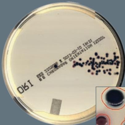
Using differential image analysis, WASPLab™ uses a preliminary colony count to group plates by CFU's, which are then presented to the reader for verification.
