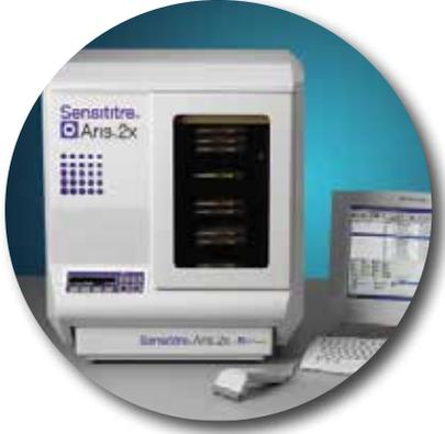
**Thermo Scientific Sensititre ARIS 2X System.** The ARIS™ 2X System is a fully automated, benchtop incubating and reading system that reduces workload and facilitates efficient workflow. It can accommodate 64 MIC, breakpoint or identification plates, for a combination of 192 possible tests on a single instrument.
