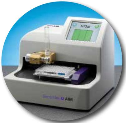
**Thermo Scientific Sensititre AIM Automated Inoculation Delivery System.** The Sensititre AIM™ System quickly and accurately doses most 96-well plates, eliminating both skipped wells and costly repeat tests.
