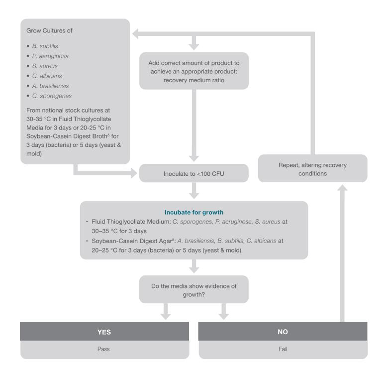
To reduce the risk of contamination during sterility testing, the procedure should be carried out in a closed system under aseptic conditions. Most organizations interpret this as using an ISO-regulated laminar airflow cabinet within an ISO-regulated clean room, or an isolator in a controlled environment.
