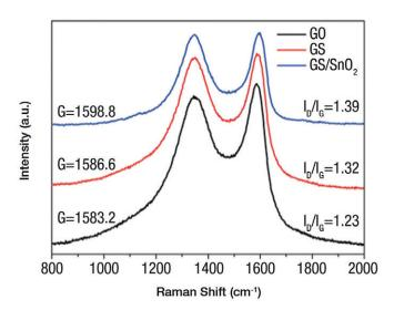
Figure 3. Hybrid anode material  $SnO_2$  and graphene sheet (GS). Comparison of the peak location of the G band between graphene sheet (GS), graphene oxide (GO), and the hybrid anode material (GS/SnO<sub>2</sub>). Raman spectra collected using a DXR Raman Microscope with a 532 nm laser. Adapted with permission from Chaohe Xu, Jing Sun, Lian Gao, J. Mater. Chem. 22, 2012, 975-979. Copyright 2012 RSC Publishing.
