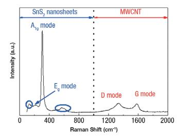
Figure 4. Raman spectrum of the SnS<sub>2</sub>/MWCNT composite material. Peaks associated with both the SnS<sub>2</sub> nanosheets and the multi-walled carbon nanotubes are observed. Raman spectra collected using a Nicolet Almega Dispersive Raman Spectrometer. Adapted with permission from Jin-Gu Kang, Gwang-Hee Lee, Kyung-Soo Park, Sang-OK Kim, Sungjun Lee, Dong-Wan Kim, Jae-Gwan Park, *J. Mater. Chem.* 22, 2012, 9330-9337. Copyright 2012 RSC Publishing.
