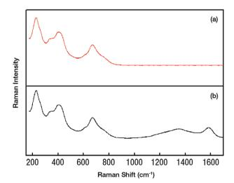
Figure 5. (a) Raman spectrum of  $\text{Li}_4\text{Ti}_5\text{O}_{12}$  and (b) Raman spectrum of carbon-coated  $\text{Li}_4\text{Ti}_5\text{O}_{12}$ . Raman spectra were obtained using a Nicolet Almega XR Dispersive Raman Spectrometer configured with a 633 nm laser. Adapted with permission from Ju Bin Kim, Dong Jin Kim, Kyung Yoon Chung, Dongjin Byun, Byung Won Cho, *Phys. Scr.* T139, 2010. Copyright 2010 IOP Publishing.
