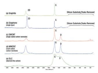
Figure 2. Raman spectra of different forms of carbon: (a) graphite, (b) single layer of graphene, (c) single-walled carbon nanotube (SWCNT), (d) multi-walled carbon nanotube (MWCNT), (d) diamond-like carbon (DLC). These spectra were obtained using a DXR Raman Microscope and a 532 nm laser.
