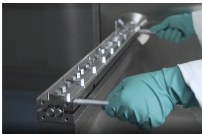
Figure 3. Twin-screw extruder split barrel design.
