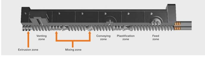
Figure 1: Barrel and screw layout.
