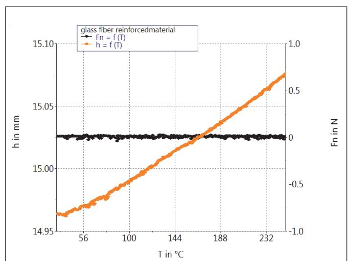
**Fig. 6:** Constant normal force (black) and increasing sample length (orange) during a temperature increase from 30 °C to 250 °C on one of the glass fiber enforced PPS samples.
