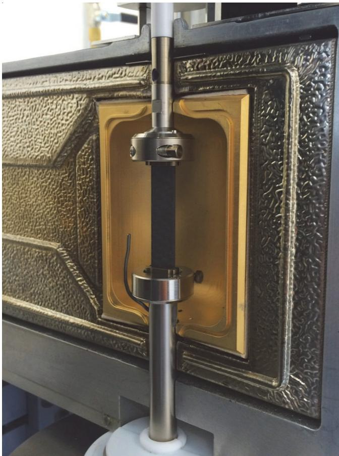
**Fig. 2:** Solids clamping tool with carbon fiber enforced composite sample.
