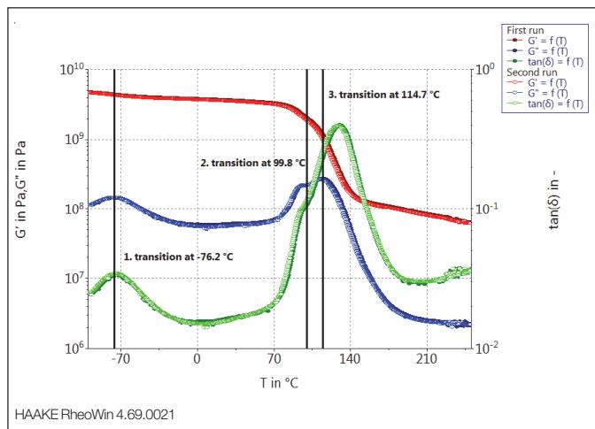
**Fig. 3:** Storage modulus  $G'$  (red), loss modulus  $G''$  (blue) and  $\tan(\delta)$  (green) as a function of temperature for the carbon based sample. The glass transition temperature  $T_g$  is indicated by the green line. The results of 2 independent tests (open and filled symbols) run on fresh samples each, show the excellent reproducibility of the results.
