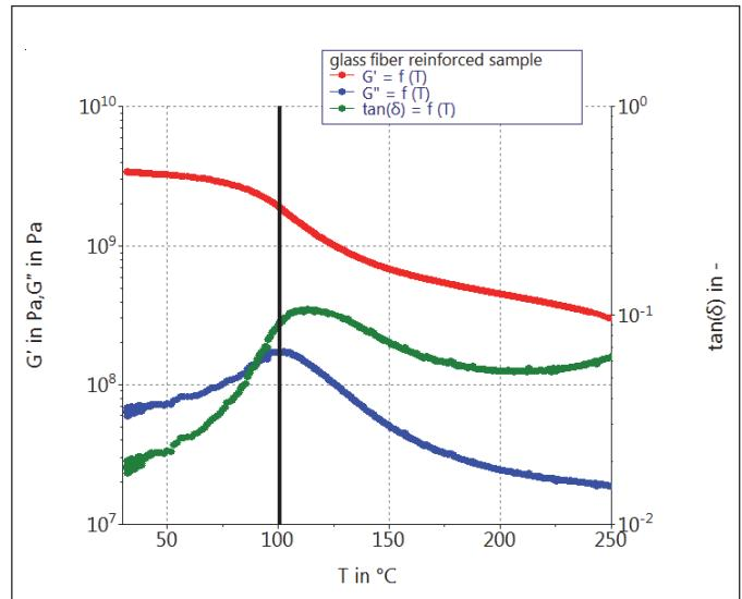
**Fig. 5:** Storage modulus  $G'$  (red), loss modulus  $G''$  (blue) and  $\tan(\delta)$  (green) as a function of temperature for a glass fiber reinforced PPS sample. The glass transition temperature  $T_g$  is indicated by the black line.
