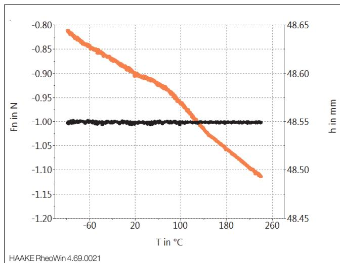
**Fig. 4:** Constant normal force (black) and decreasing sample length (orange) during a temperature increase from -100 °C to 240 °C on the carbon fiber enforced sample.
