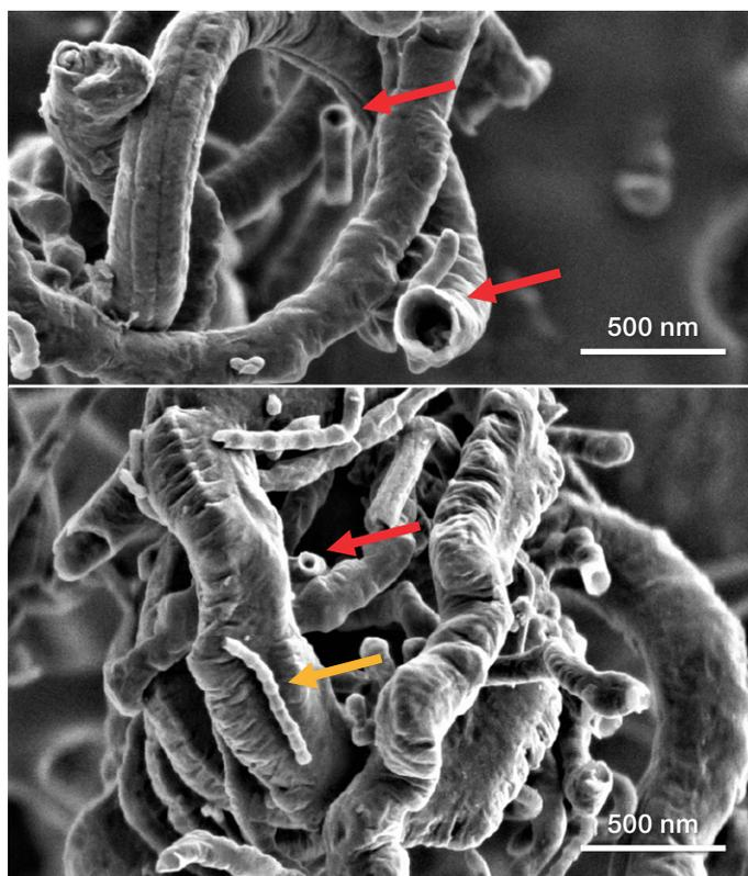
Figure 2. Higher magnification images of carbon nanotubes. Acc voltage 1 keV, beam current 6.3 pA. Red arrows in images show the inner part of the carbon nanotubes. The yellow arrow points to the characteristic shape of a bamboo-like carbon nanotube.
