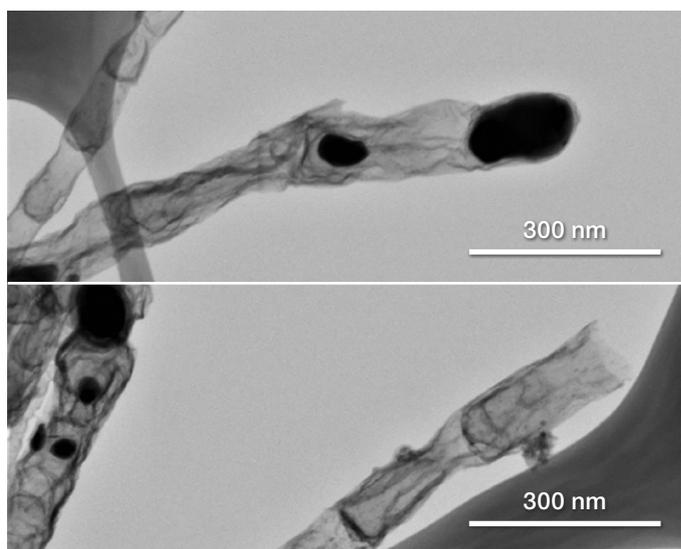
Figure 7. Bright field images of characterized bamboo-like carbon nanotube ends. Top image shows a closed end with an  $\approx 5$  nm layer on an elongated catalyst particle. Bottom image shows an open end.
