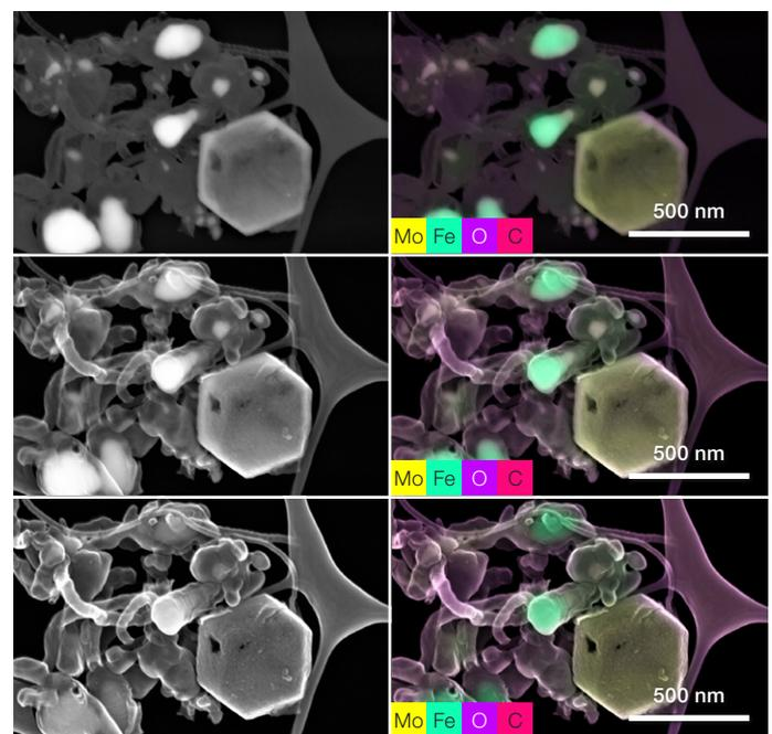
Figure 4. T1, T2, T3 images of a group of nanotubes with particles of different contrast. (left) Grayscale images. (right) Related ChemiSEM Technology images show iron-rich presence of the catalyst particles and an unexpected material rich in molybdenum and oxygen.
