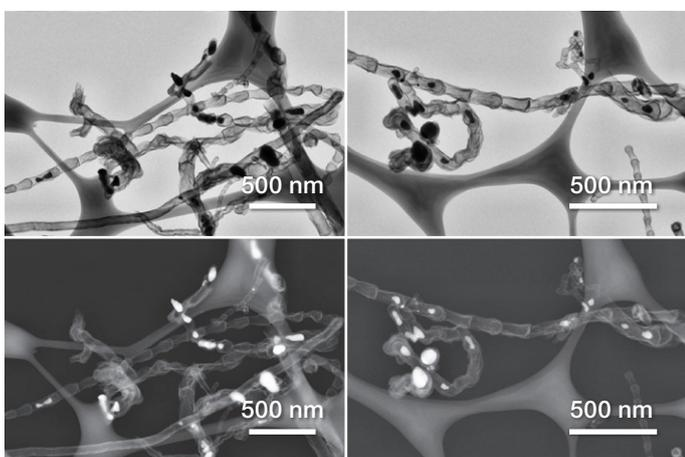
Figure 6. Bright field and high angle annular dark field images. Using an accelerating voltage of 30 keV and a beam current of 6.3 pA, (top row) BF images and (bottom row) HAADF images show the bamboo-like structure, distribution, and shape of the catalyst particles.
