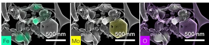
Figure 5. ChemiSEM Technology images showing distributions of elements of interest. From left to right, images show respectively the distribution of iron, molybdenum and oxygen.
