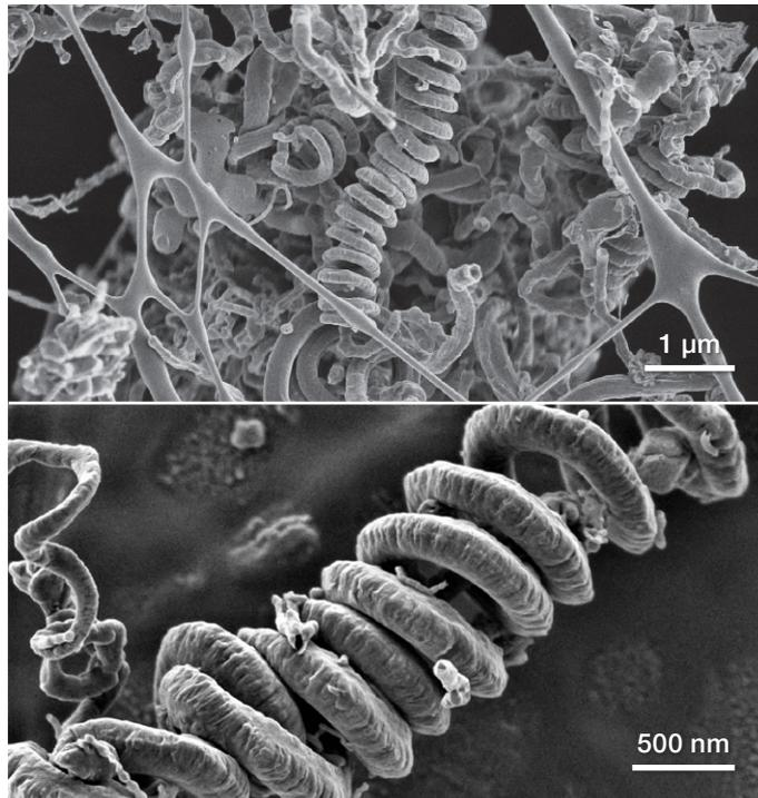
Figure 1. Overview of the different carbon nanotubes. Both (top and bottom) images show the tubes' morphology and surface roughness. Acc voltage 1 keV, beam current 6.3 pA.
