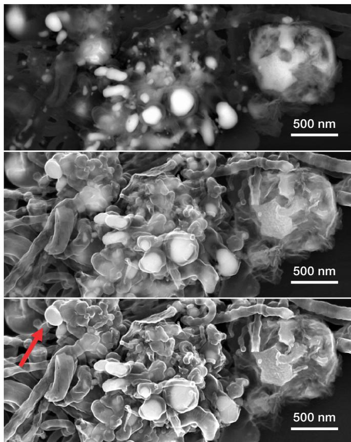
Figure 3. Set of three images simultaneously acquired using the Apreo 2 SEM and in-column Trinity Detection System. Using an accelerating voltage of 15 keV and a beam current of 0.2 nA, top image was acquired with a T1 detector, middle image was acquired with a T2 detector, and bottom image was acquired with a T3 detector.
