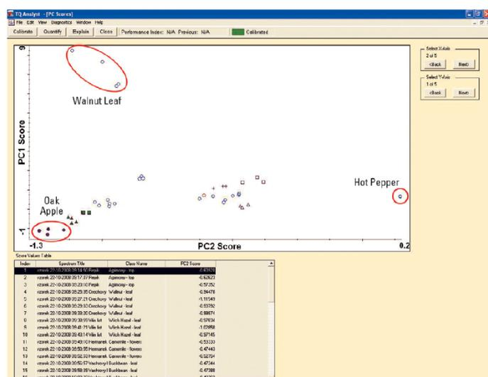
Figure 4. Principal component score plots showing class clustering as a function of the first and second principal components. Heterogeneous samples tended to have widely scattered clusters (walnut leaf, oak apple), while homogeneous samples were tightly clustered (hot pepper). Clusters were well defined and there were no overlapping clusters for the classes when viewed in 5-dimensional principal component space.
